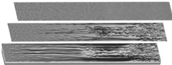
POD used to extract important flow structures
