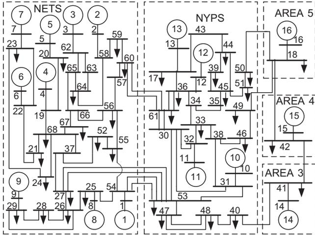
Fig. 13. NETS–NYPS test system.
