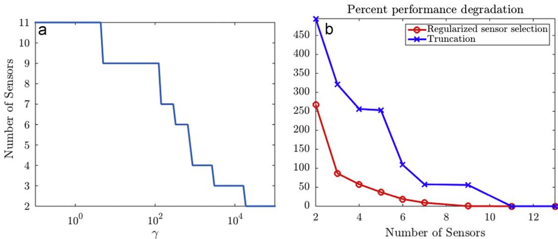
Fig. 12. (a) Number of sensors as a function of the sparsity-promoting parameter  $\gamma$ ; and (b) performance comparison of the Kalman filter associated with the sets of sensors resulting from the regularized sensor selection problem and from truncation.
