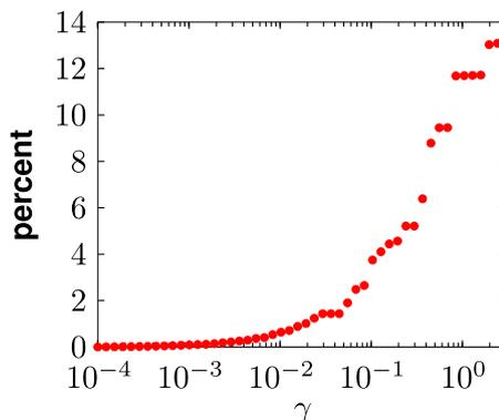
Fig. 15. Performance vs. sparsity ( $(J - J_c)/J_c$  vs.  $\text{card}(F)/\text{card}(F_c)$ ) comparison of sparse  $F$  and the optimal centralized controller  $F_c$  for 50 logarithmically spaced points  $\gamma \in [10^{-4}, 3]$ .
