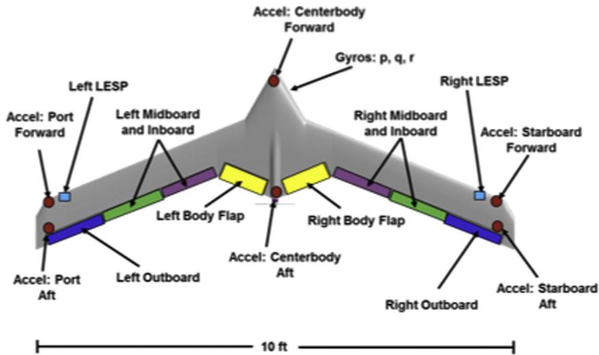
Fig. 11. Body Freedom Flutter flexible wing testbed aircraft.
